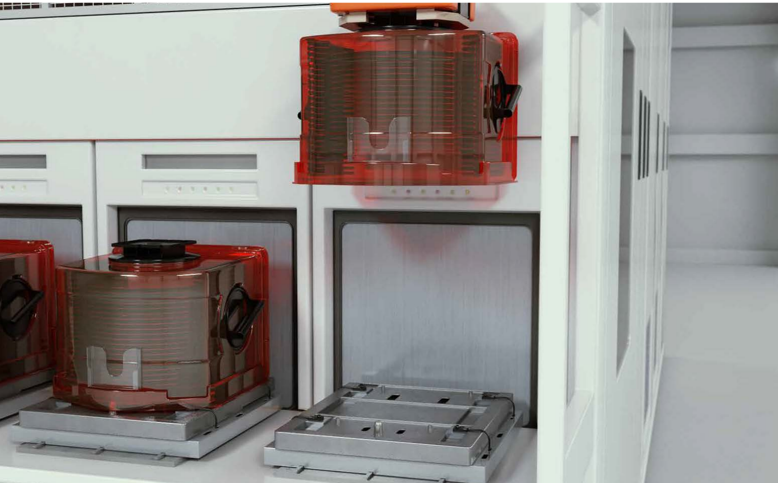
Photomicro sensors are used to detect whether wafer carriers are mounted on trays to be moved into the equipment.
