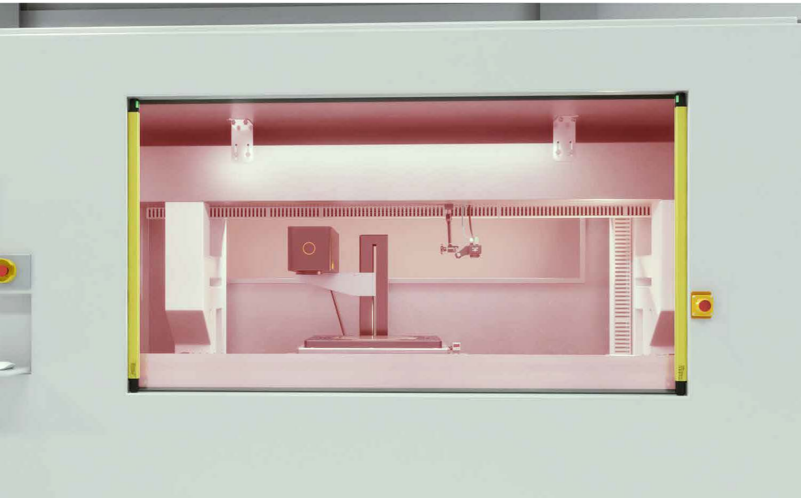
Safety light curtains can be used to detect human access to hazardous areas while equipment is operating.
