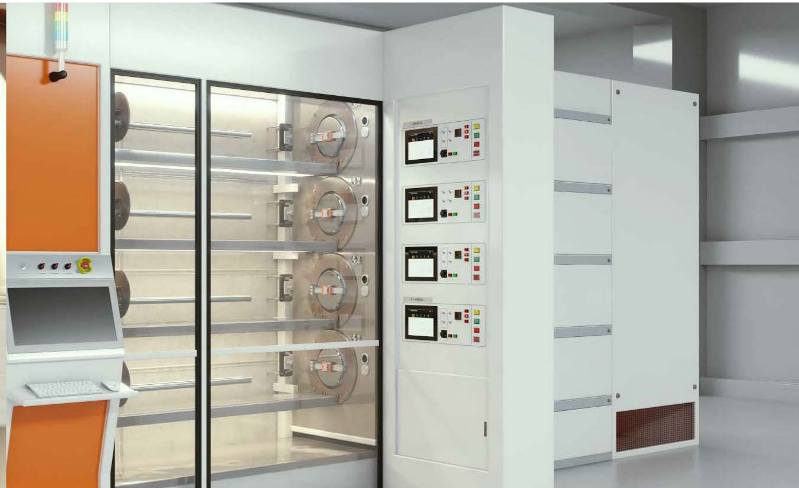
Graphic panels are used to control settings and monitor status of horizontal furnace equipment.
