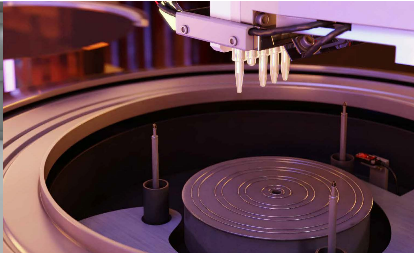
Photoelectric sensors located at the bottom of the spin coater are used to detect whether wafer is mounted before applying the solution.
