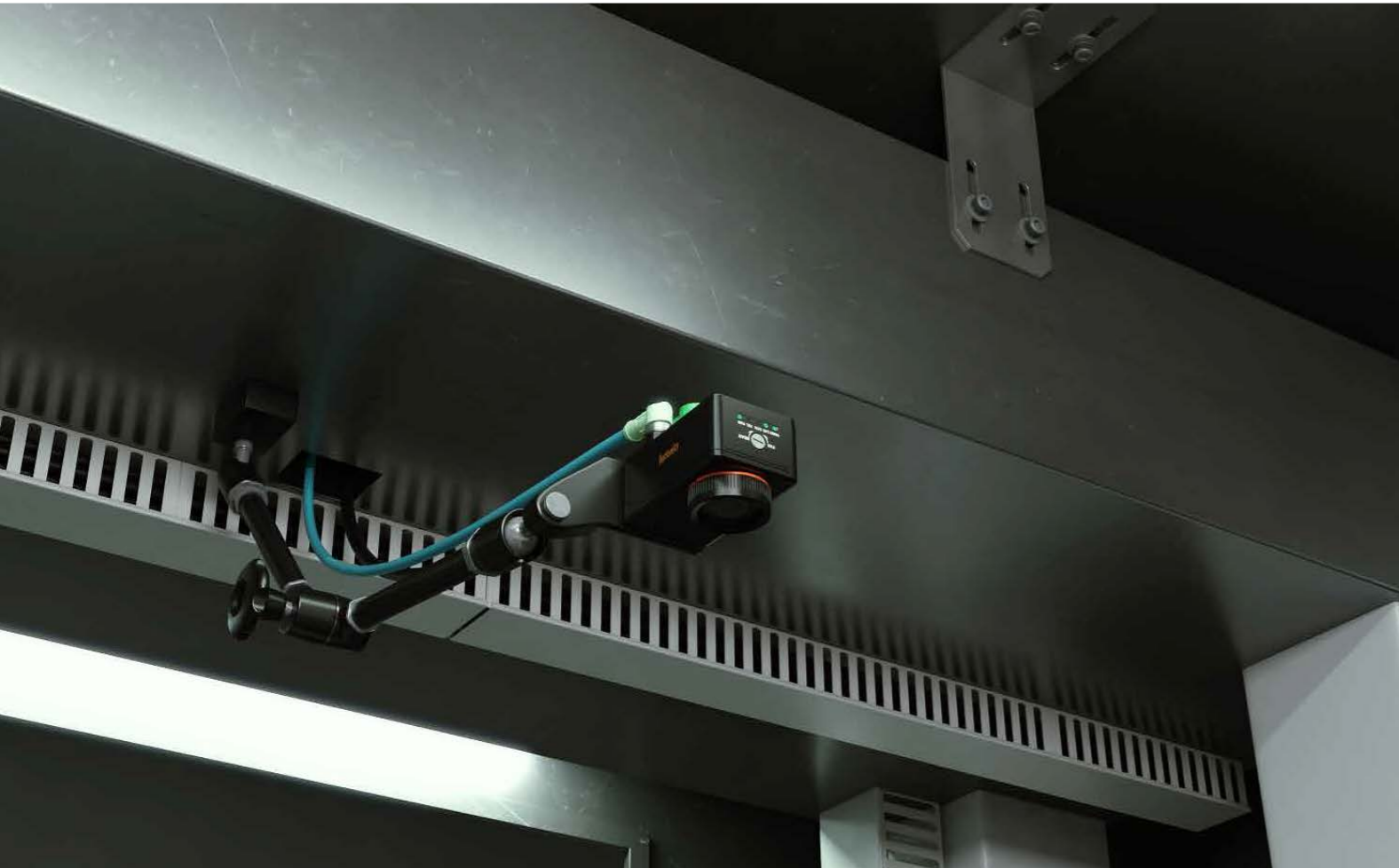
Vision sensors are used to check presence and status of laser marking on wafers.
