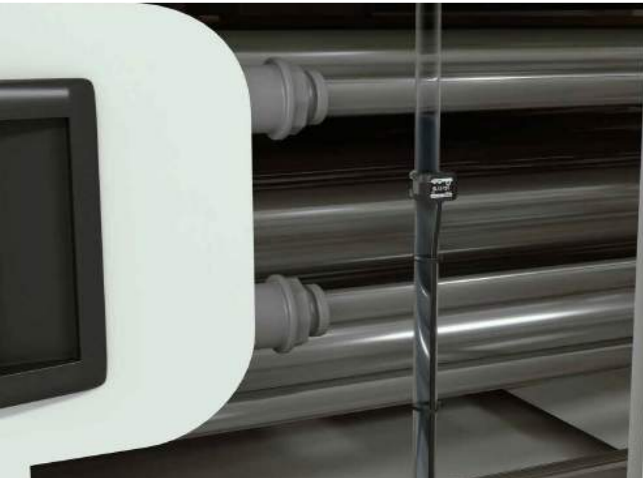
Liquid level photoelectric sensors are used to detect the amount of cleaning fluid in the cleaning equipment.
