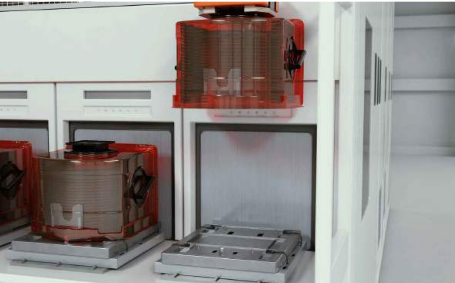
Photomicro sensors are used to detect whether wafer carriers are mounted on trays to be moved into the equipment.
