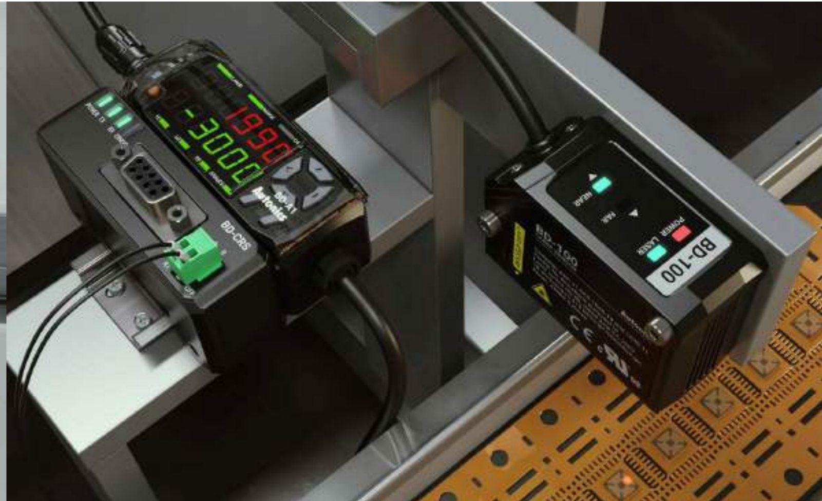
Displacement sensors can be used to detect the height change of attached chips while attaching chip cut from wafer to the PCB.
