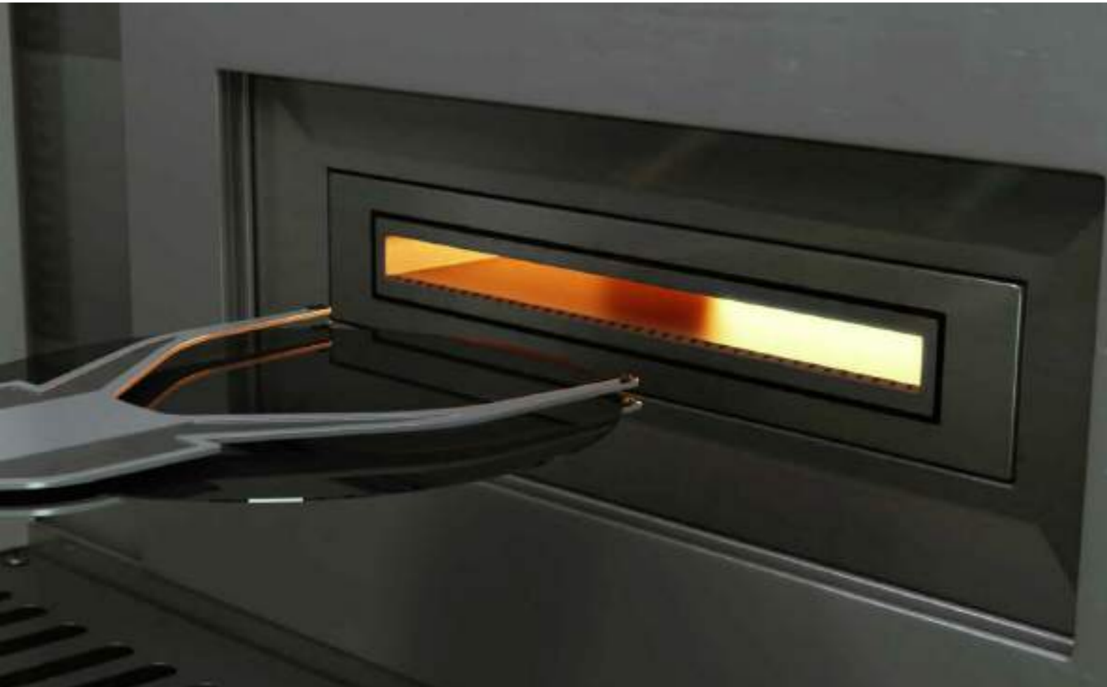
Temperature controllers are used to control the temperature of the heating device used to remove metal contaminants on wafers by applying heat.
