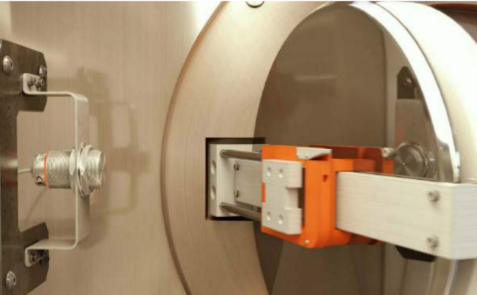
Proximity sensors are used to control the movement of wafer boat and robot arms by detecting the opening of wafer chamber door on the horizontal furnace equipment.
