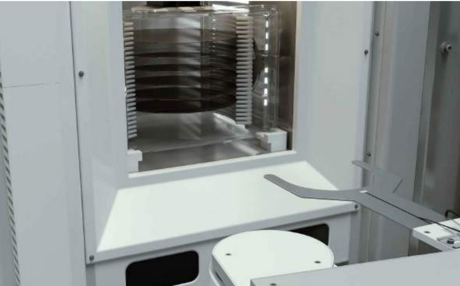
Fiber optic units are used to detect whether wafer is settled on the handler equipment for wafer taping before grinding.
